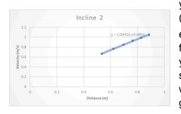
y-axis. The equation that this linear graph projected (which directly represents and matches the simplified equation of  $V=\sqrt{2a} \times \sqrt{\Delta X}$ ) is y=.8196x+.0025 for the first instance where the inline is 3.8 meters and y=1.0942x+.0856 for the inline of 7.8 meters for the second instance. Using the slope from these equations, we then could solve for acceleration using the equations given.
